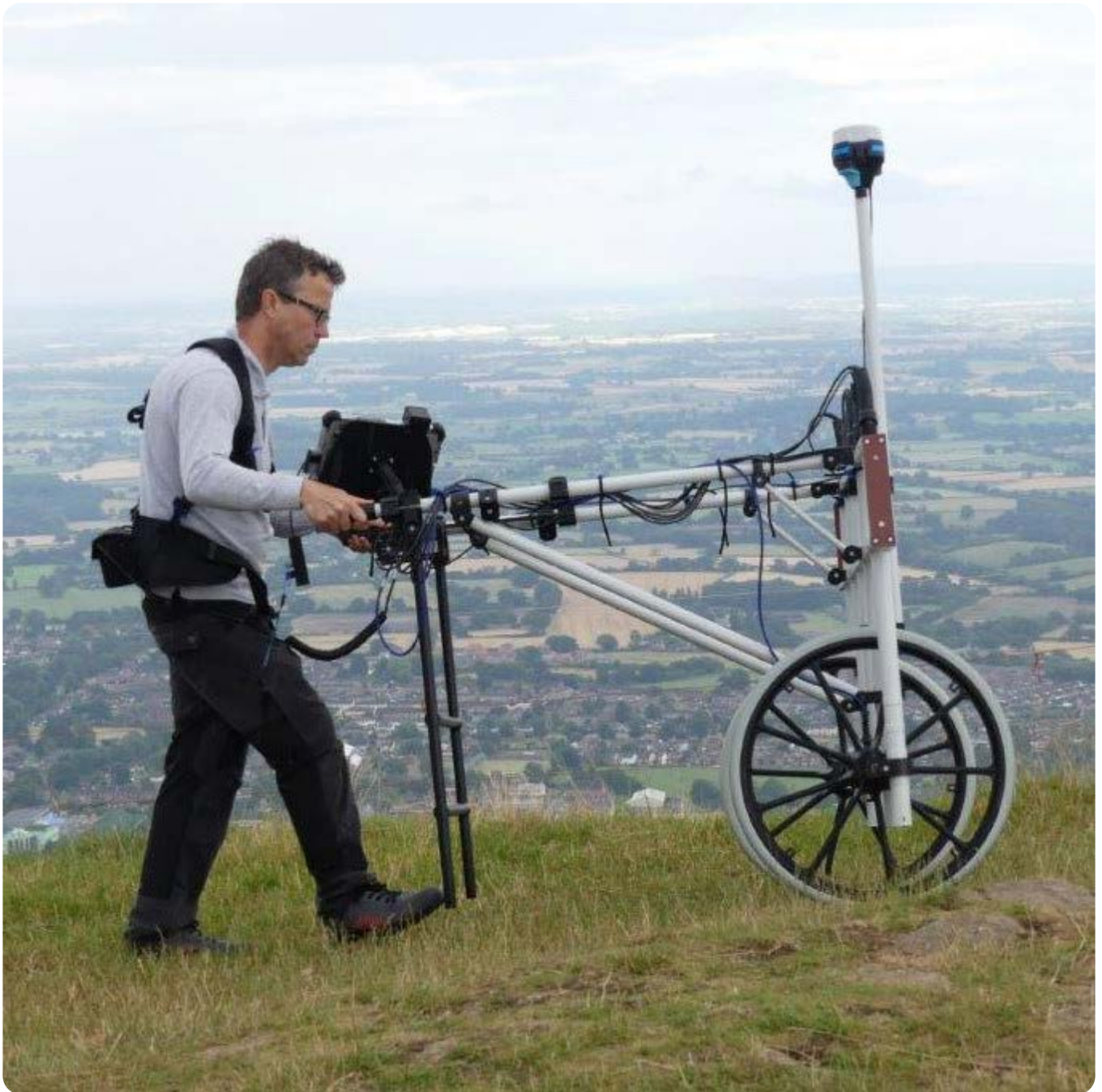
Data Collection with a magnetometer, Malvern Hills.
