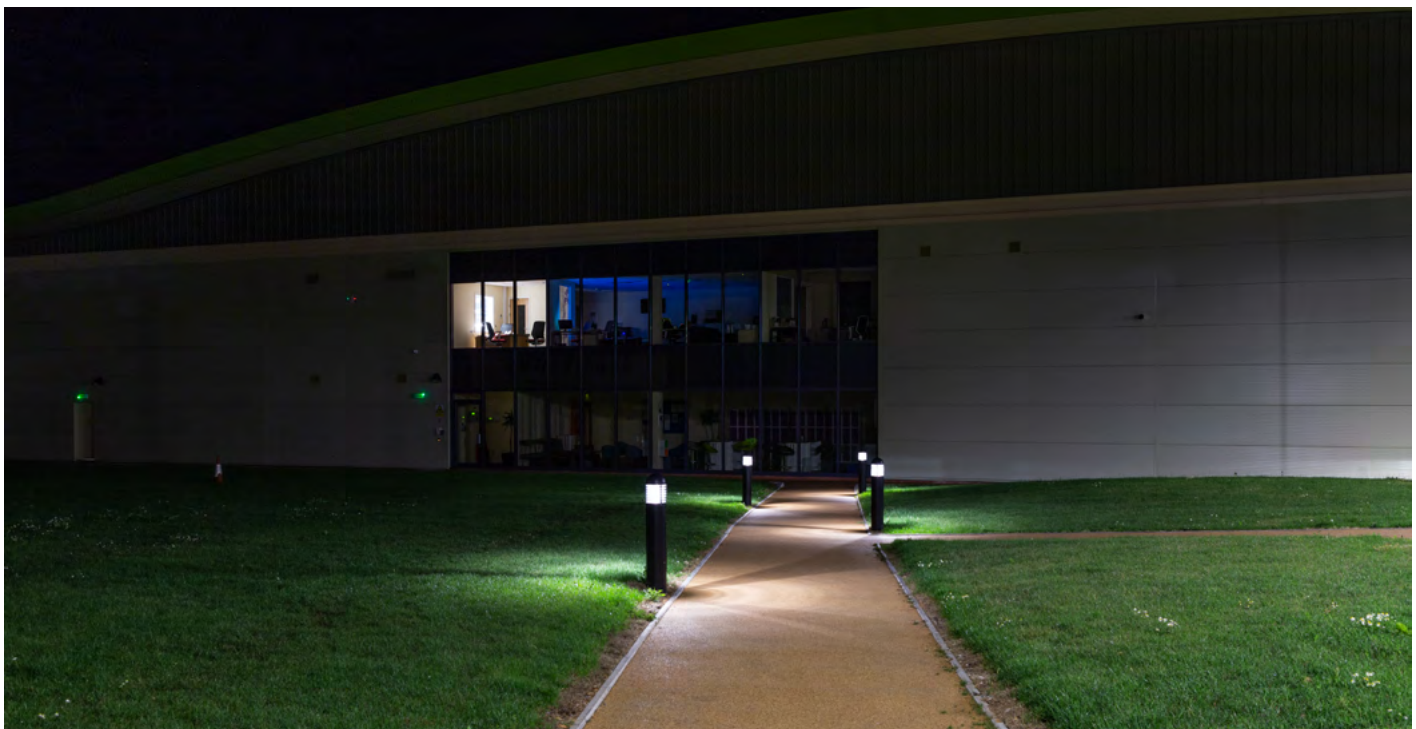
Figure 40 - Path edge bollards produce just enough light to mark routes and are sparingly used throughout the site. © Malvern Hills NL Team
