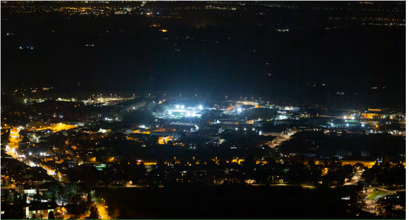
Figure 20 – Malvern development. Note the higher white colour, glare, and upward light compared to the street lighting.
