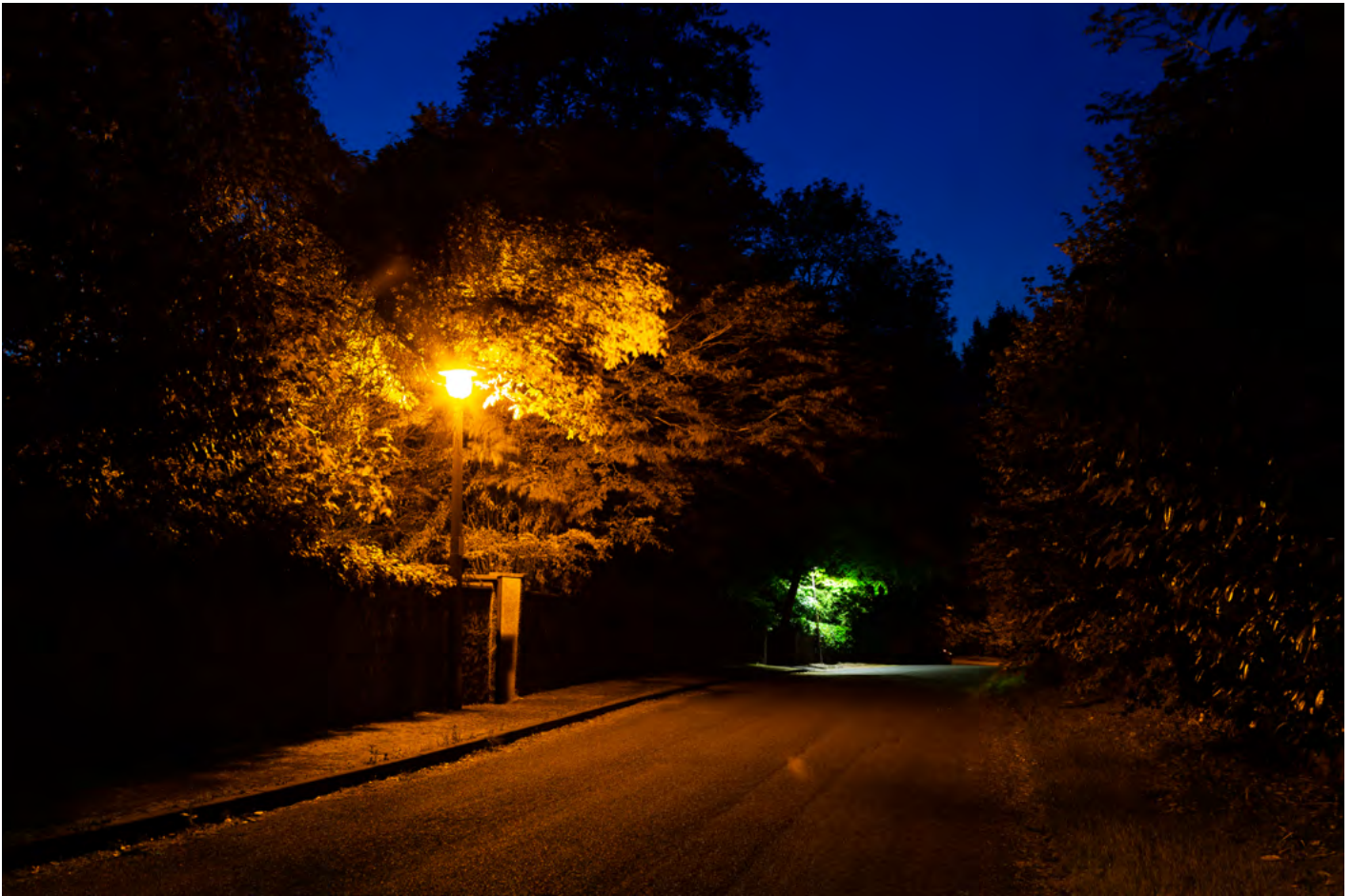
Figure 38 - Contrast between old style sodium street light in foreground and new LED light in background © Malvern Hills NL Team
