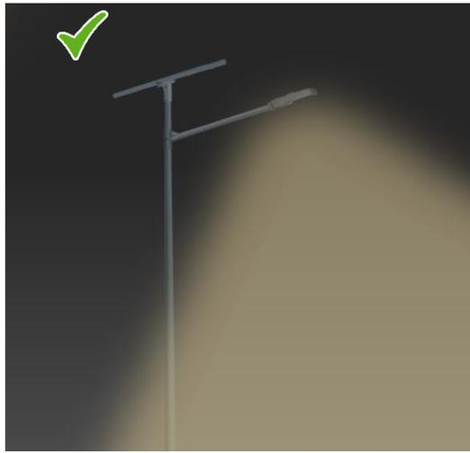
6.48 White luminaires with a high amount of upward light should be avoided. Even with heritage area needs, street lighting should <math><3000\text{K}</math> and direct light downward.
