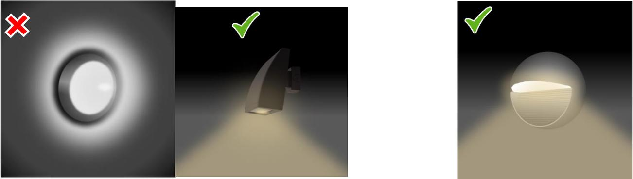
6.13 Avoid circular bulkhead lights that emit light upward. Use bulkhead lights that direct light downwards or have shielding. Try and ensure that emergency luminaires on batteries follow these principles.
