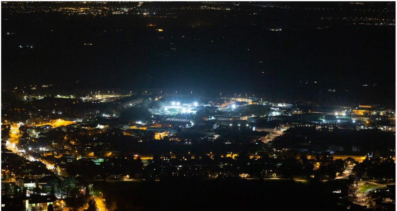
Figure 20 – Malvern Hills Science Park. Note the higher white colour, glare, and upward light compared to the street lighting.
