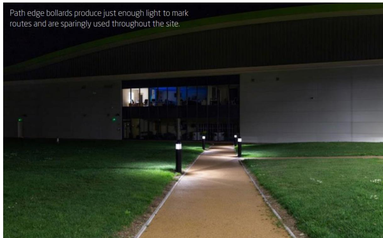
*Figure 33 - Path bollards*
