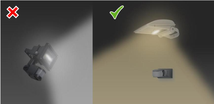
5.11 Avoid halogen security lights with a fixed PIR sensor, as they cannot be tilted sufficiently and detect movement. Use tiltable lights with separate PIR Sensor so you can position the triggering point and tilt the luminaire properly.
