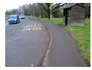
4. Crossing of junction between Worcester Road and Madresfield (northern arm). Good visibility here, but could consider tightening turn-radii of junction in order to reduce vehicle speeds. Consider painted treatment on the carriageway surface to indicate cycle route crossing.
