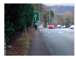
2. Crossing of junction between Worcester Road and Madresfield (southern arm). Reasonably good visibility here, but could consider tightening turn-radius of left-turn out of Madresfield in order to reduce vehicle speeds. Consider painted treatment on the carriageway surface to indicate cycle route crossing.
