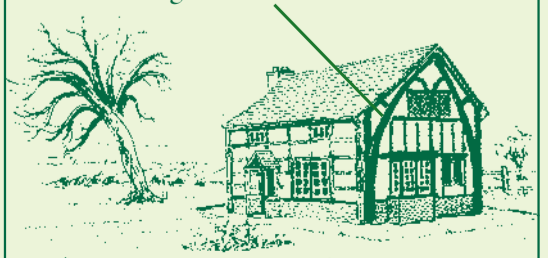
A typical 'cruck' framed House
